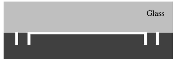
(c) High Aspect Ratio etching using  $\text{SF}_6$  and  $\text{C}_4\text{H}_8$  followed by bonding the processed side of Si wafer to Borosilicate Glass
