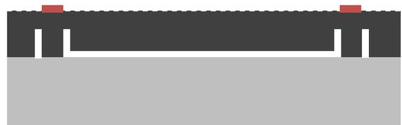
(d) Electrical contact definition by Aluminum sputtering, patterning and annealing
