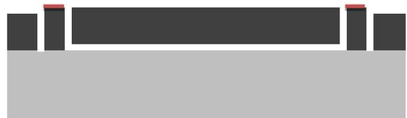
(e) Final release of the structure with  $\text{SF}_6$  and  $\text{C}_4\text{F}_8$  plasma etching
